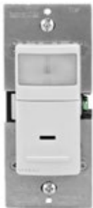
Sensor Universal 120V~ 60Hz 180° PIR Auto ON* 150W LED | CFL 300W Incand. 1/6 hp 2.5A 1P encendido relay requiere tierra Cat. IPS02
