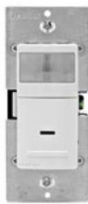
Sensor Universal 120V~ 60Hz 180° PIR Auto ON* 150W LED | CFL 600W Incand. 1/6 hp 5A 1P encendido relay requiere tierra Cat. IPS05
